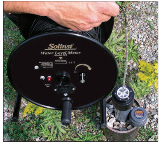
Measure Water Levels within the narrow channels of a Solinst CMT® System.
