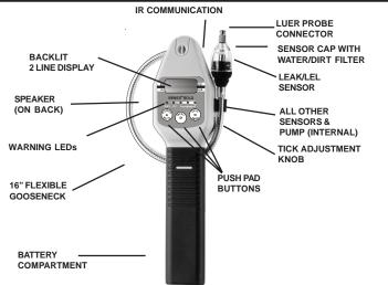
**Sensit®Gold** instruments are constructed of durable ABS plastic to withstand the rigors of field use.
