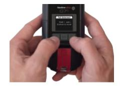
Red alerts are immediately communicated to monitoring personnel. Read the information on your G7 screen. Press and hold the up and down arrow buttons at the same time to mute the sound and vibration. This does not cancel the red alert sent to monitoring personnel.
