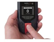
If you are safe, push the red latch button. If you do not push the latch within the configured amount of time, your yellow pending alarm will communicate a red alert to monitoring personnel.
