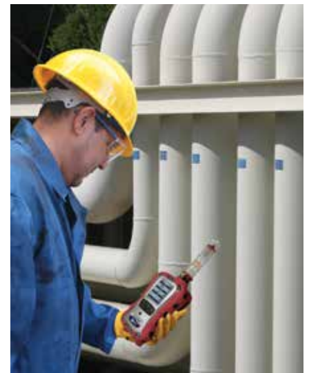
MultiRAE Benzene used for leak detection
