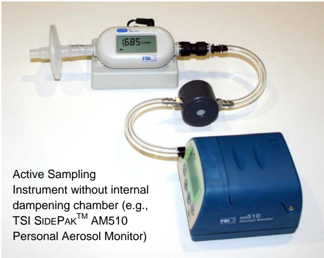
Figure 2-3 Typical Dampening Module Set Up
