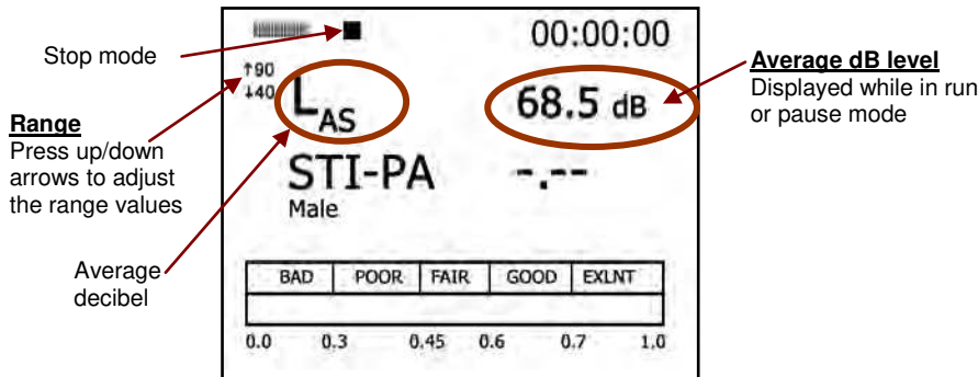
Figure 6-20: Level set-up and average decibel level
