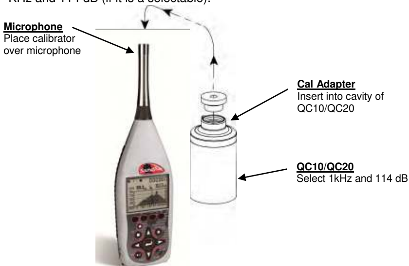
Figure 5-2: Attaching calibrator to SoundPro
