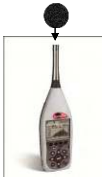
Figure 2-3: SoundPro with microphone and windscreen
