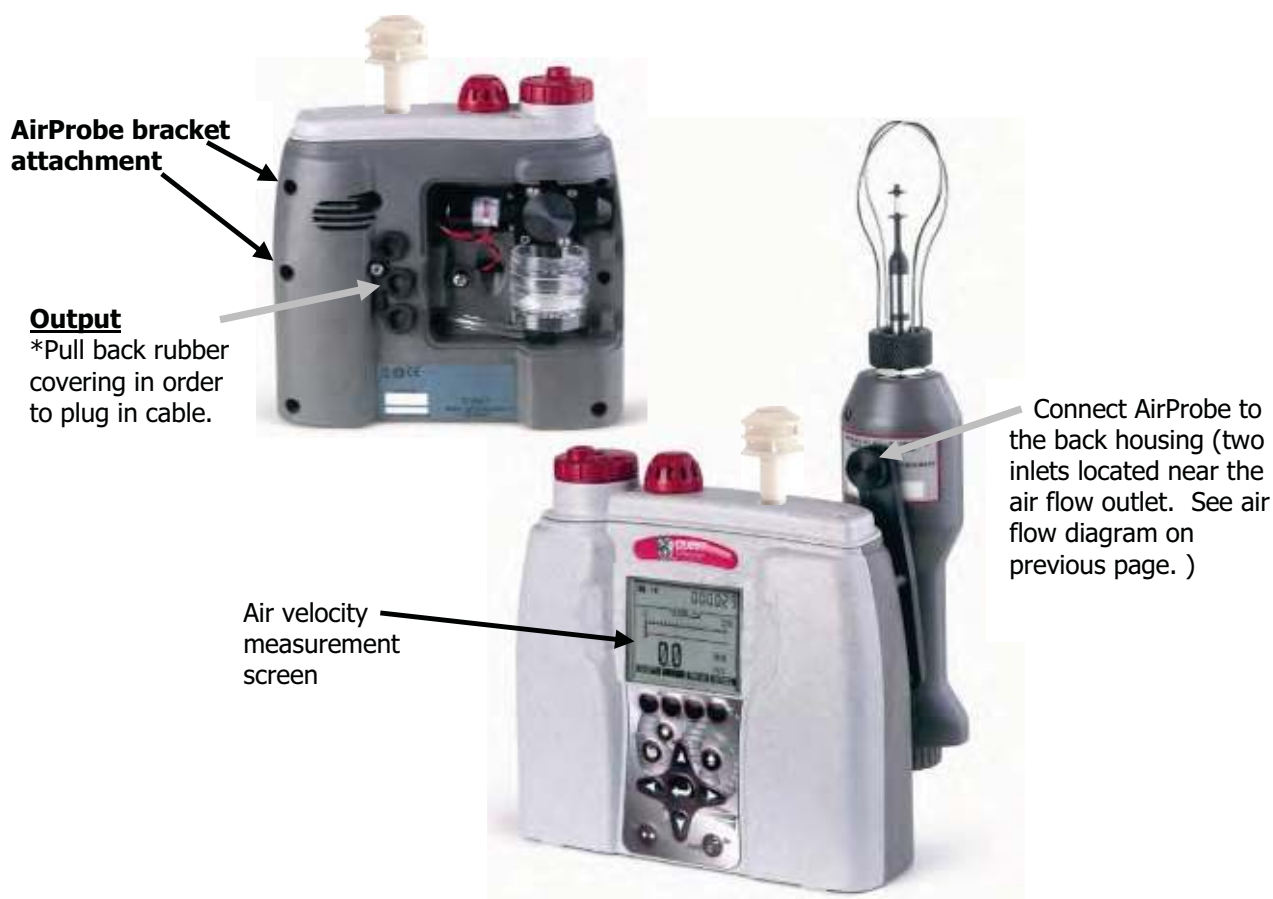
Figure 5-11: Attaching AirProbe and measuring Air velocity
