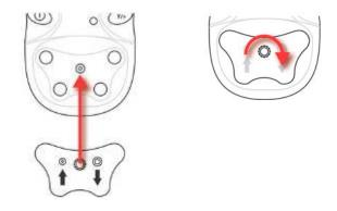
**Note:** Finger-tighten this only. Do not use pliers or other tools. The Calibration Adapter should be snug, but an air-tight seal is unnecessary.
