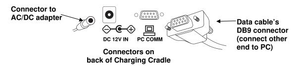
The QRAE II's cradle connects via a DB9 (9-pin) connector to a computer running ProRAE Remote software.
