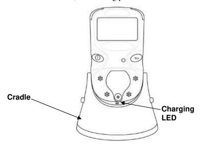
**Note:** Before setting the QRAE II into its charging cradle, visually inspect the contacts to make sure they are clean. If they are not, wipe them with a soft cloth. Do not use solvents or cleaners.
