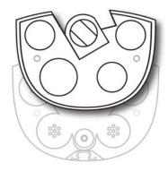
6. Turn over the plate holding the pump, and lift the pump off.
