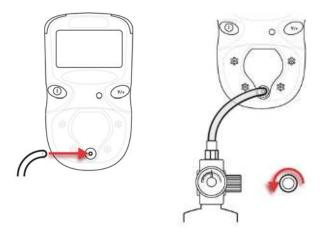
3. After calibration, turn off the gas and remove the hose from the QRAE II Pump.
