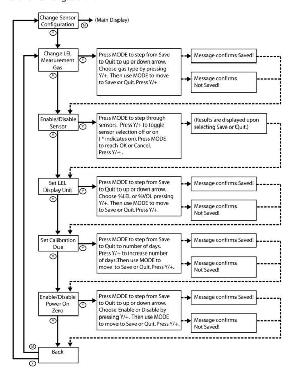
**Change LEL Measurement Gas.** This function allows selection of the measurement gas for the LEL sensor. The correction for the measurement gas is automatically divided by the correction factor the span gas, selected previously, to obtain a new factor for the combination of gases. The new factor is applied to the readings to obtain a true concentration.
