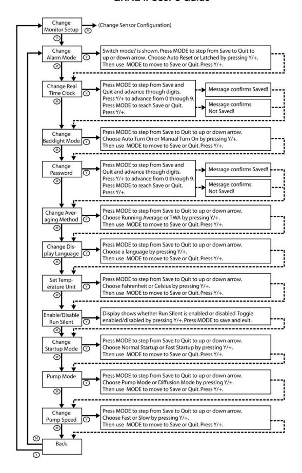
**Change Alarm Mode.** Your choices are Auto Reset and Latched. A latched alarm stays in alarm until you acknowledge the alarm by pressing a button. An auto-reset alarm turns off when the condition that set off the alarm is no longer present (for instance, a high H2S reading that exceeds the preset threshold and triggers an alarm, but then lowers below that threshold, turning the alarm off).
