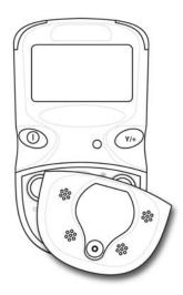
5. Turn over the cover and pull off the plate with the pump attached.
