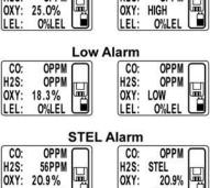
Low Alarm: Buzzer, LED: 2 times/second Vibrator: 400ms/second
