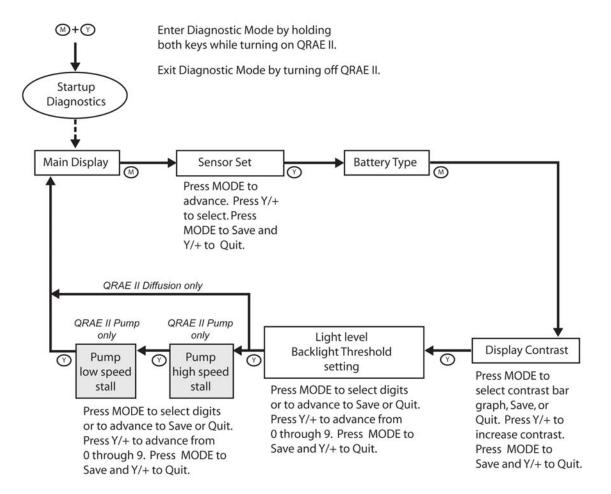
**Sensor Set.** Two sensor options are available. When any sensor is exchanged for another type, the firmware must be set to match the sensor. The upper right sensor slot can accommodate either a CO sensor or an  $SO_2$  sensor. The upper left sensor slot accommodates an  $H_2S$  0.1-100 ppm sensor.
