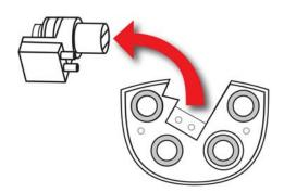
7. Replace the pump by pressing the new pump firmly into its recessed area on the plate.
