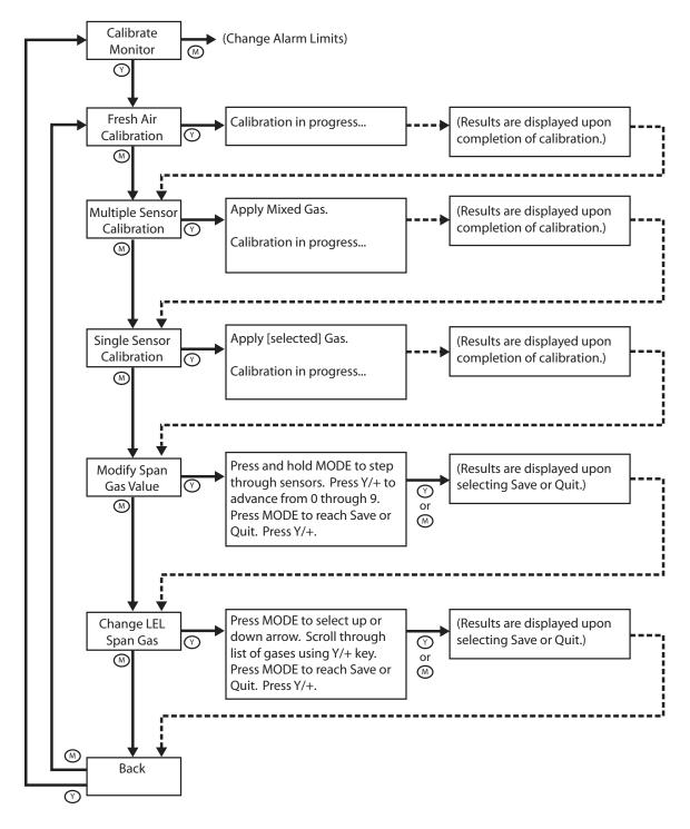
**Fresh Air Calibration.** This sets the zero point of the sensor calibration curve for clean air. Expose the inlet to a clean air source with 20.9% oxygen and without any organic, toxic or combustible gas impurities. Follow the procedure outlined in "Zero (Fresh Air) Calibration" on page 49.
