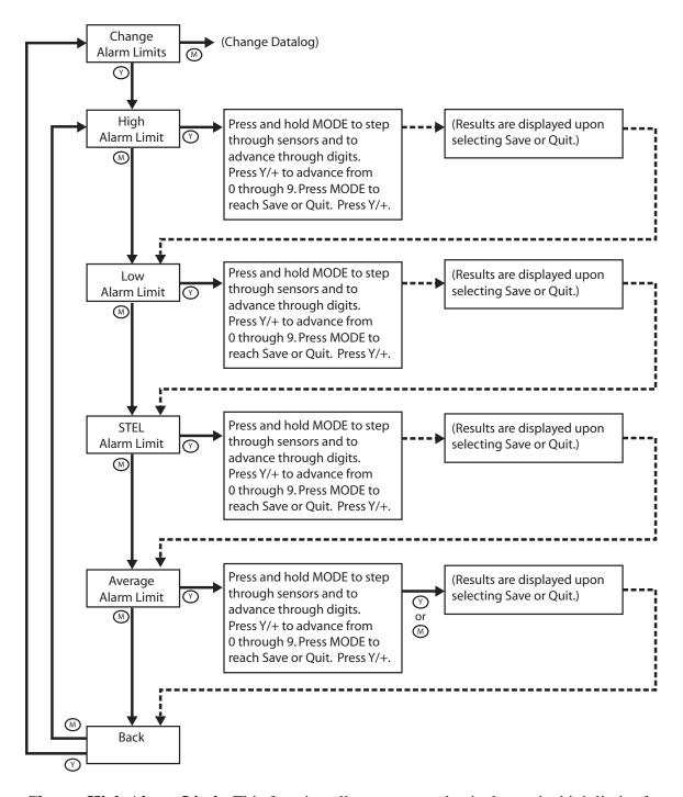
**Change High Alarm Limit.** This function allows you to selectively set the high limit of individual sensors in the QRAE II.
