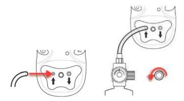
**Caution!** After calibration is complete, remove the Calibration Adapter. When monitoring, never operate the QRAE II with the Calibration Adapter attached. The QRAE II's sensors operate by diffusion. If the Calibration Adapter is attached during normal operation, inconsistent and lower-than-normal readings will occur because of decreased concentration of the gas being monitored.
