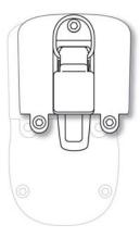
3. Hold the QRAE II down and lift the compartment cover by pulling on the belt clip.
