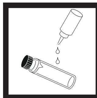
**3.** Apply a thin film of silicone oil. Wipe with a soft cloth to obtain an even film over the entire surface.
