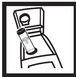
9. Thoroughly mix the 90 to 110 NTU standard, then fill a clean sample cell to the line with the standard. Insert the cell into the cell compartment.
