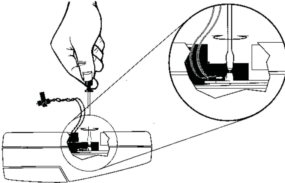
6. Hold the new lamp assembly by the tab with the lamp facing the top (keyboard) of the instrument. Slide the small catch on the other side of the assembly into the black plastic slot (towards the nearest edge of the instrument).
