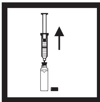
**2.** Slowly apply the vacuum by carefully pulling the plunger upward, then holding it. If using a hand or electric pump, connect the tubing to the vacuum pump with vacuum hose. Apply vacuum until visible gas bubbles disappear. **Slowly** release the vacuum. Remove the vacuum apparatus and cap the cell.
