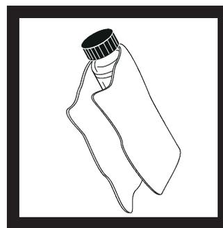
**3.** Using a soft, lint-free cloth, spread the oil uniformly, then wipe off the excess so that only a thin coat of oil is left. The cell should appear nearly dry with little or no visible oil.
