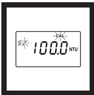
**10.** The display will show the **S2** icon (with the **2** flashing) and **100 NTU** or the value of the S2 standard for the previous calibration.
