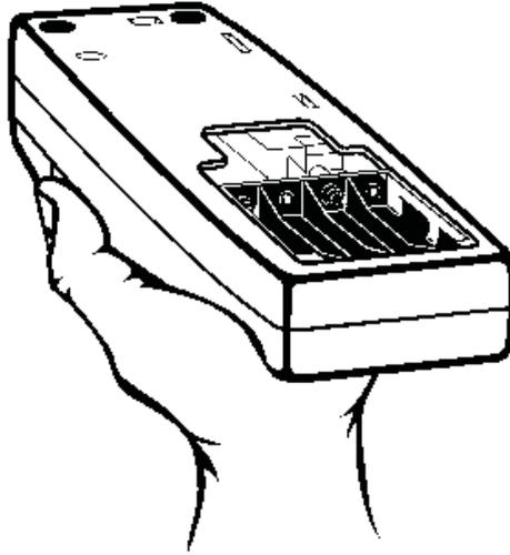
2. Remove the lamp assembly by grasping the tab on the left side of the assembly. Firmly, but gently, slide the assembly towards the rear of the instrument.
