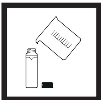
**1.** Collect a representative sample in a clean container. Fill a sample cell to the line (about 15 mL), taking care to handle the sample cell by the top. Cap the cell. (See *Section 2.3* on page 22 for more information about collecting a representative sample).
