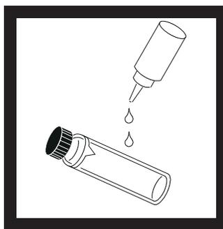
**2.** Apply a small bead of silicone oil from the top to the bottom of the cell-- just enough to coat the cell with a thin layer of oil.
