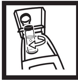
**8.** Remove the cell, rotate it slightly and reinsert into the cell compartment. Close the cover, then press **READ** again. Record the cell's position and the displayed reading.
