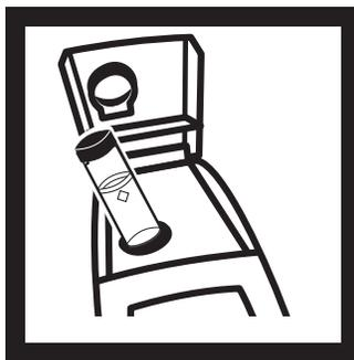
**2.** Insert the sample cell in the cell compartment by aligning the orientation mark on the cell with the mark on the front of the cell compartment. Close the lid. Press I/O.
