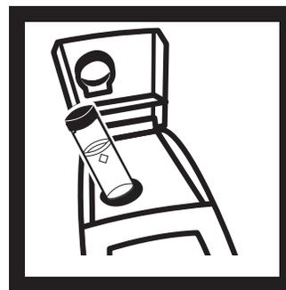
**6.** Insert the **second** sample cell into the cell compartment and close the cover.
