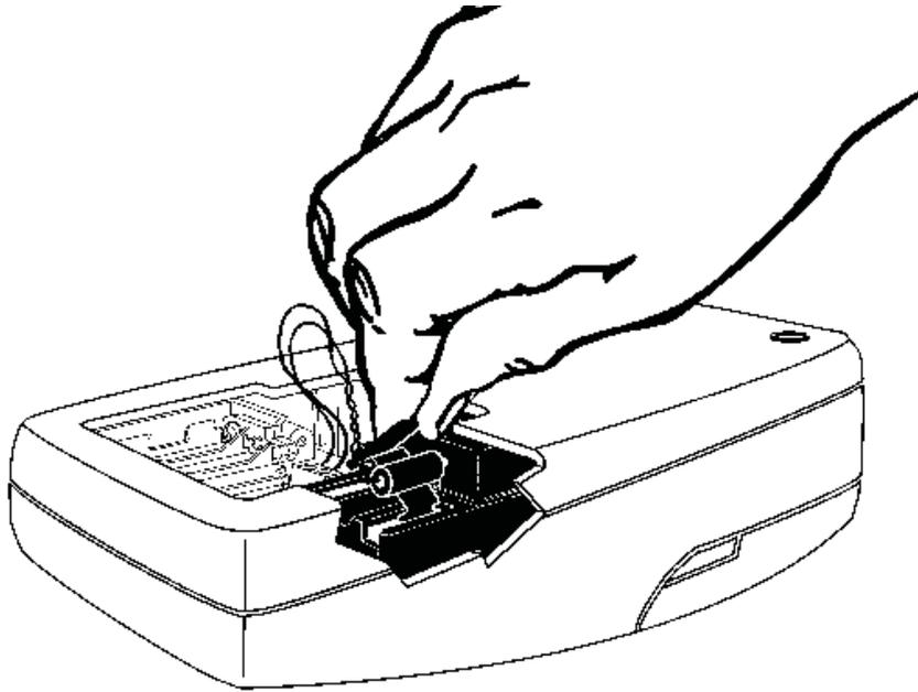
4. Back the terminal block screws **partially** out (1 to 2 turns) and remove the old lamp leads.
