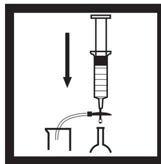
3. Draw about 50 mL of sample into the syringe. Slowly push on the plunger to force the water through the filter and into a graduated cylinder or volumetric flask. Repeat Steps 2 and 3 until the desired amount of water is obtained.
