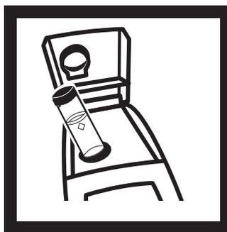
5. Insert the sample cell in the instrument cell compartment so the diamond or orientation mark aligns with the raised orientation mark in front of the cell compartment.
