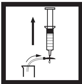
2. Fill a beaker or container with the water to be filtered. Insert the tubing into the container. Slowly draw the water into the syringe by pulling up on the syringe plunger.
