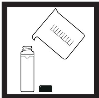
**1.** Fill a clean sample cell to the line (about 15 mL) with dilution water.
