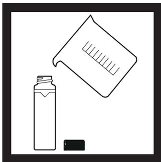
**1.** Rinse a clean sample cell with dilution water several times. Then fill the cell to the line (about 15 mL) with dilution water or use StablCal <math><0.1</math> NTU standard.
