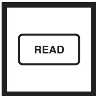
**16.** When all the digits show the appropriate value, press **READ**. The instrument will count from 60 to 0 (67 to 0 if signal average is on), measure the turbidity and store the value. The instrument will increment back to **S0**. Remove the sample cell from the cell compartment.
