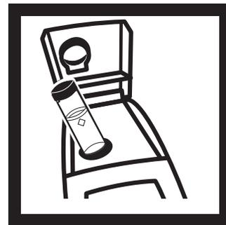
6. Repeat *step 3* through *step 5* for the other Gelex standards, being careful to orient the cells properly.
