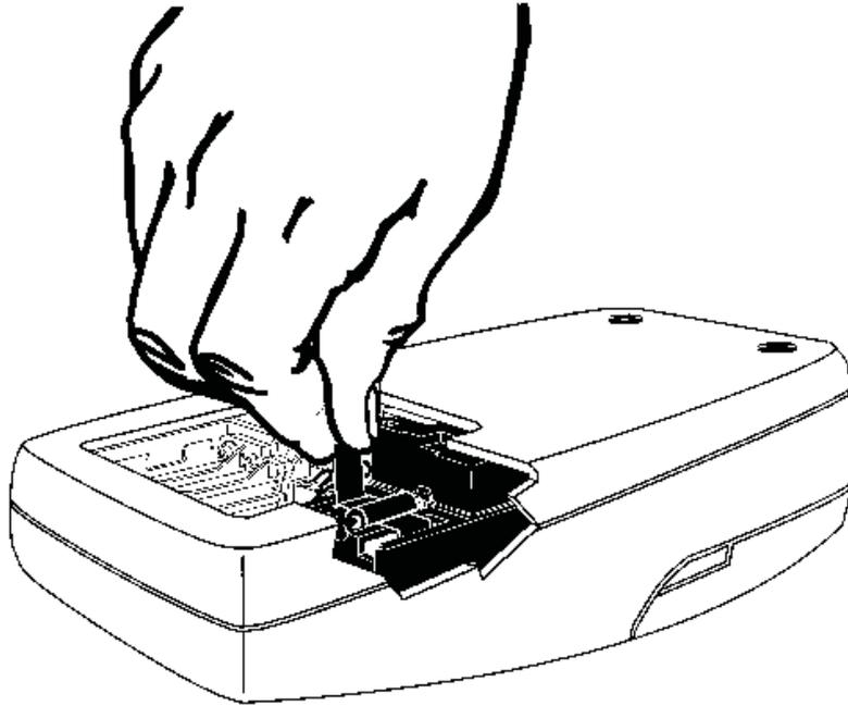
8. With your thumb, firmly slide the assembly forward until it stops. Again, push firmly against the tab to make sure the lamp is seated correctly.
