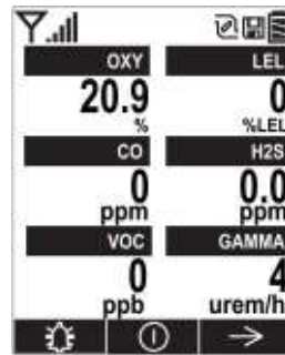
Six-threat configuration with CO+H2S combo sensor
