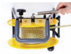
Figure 2 To Test the Entire System: Make sure sensitivity dial is turned fully clockwise. Touch the probe body to the standoff screw and probe tip to the stud (on axle) at the same time. The buzzer will sound if the system is okay.
