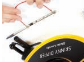
Figure 2 To Test the Entire System: Make sure sensitivity dial is turned fully clockwise. Touch one end of a conductive wire to the probe body and the other end to the last weight. This will create a short in the probe, the buzzer will sound if the system is okay.
