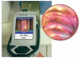
CCD camera and small-spot feature isolates and stores small sample area measurements.
