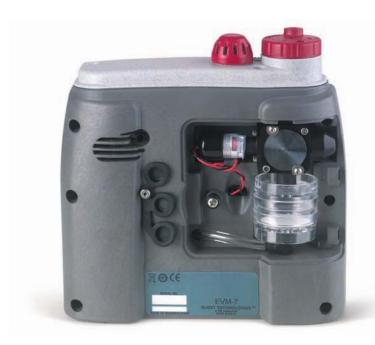
Removal of the back cover allows for convenient access and customization of gravimetric filter cassette for sample collection.
