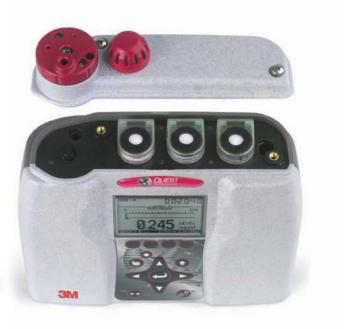
Removable sensor bar provides easy access to toxic electrochemical sensors.
