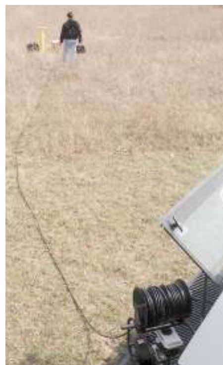
The optional Cart Kit (top photo) and 200' Air Hose Reel (bottom) greatly increase the sampling range and versatility of the basic MP40 Compressor.
