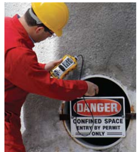
Confined space testing with the MultiRAE Lite
