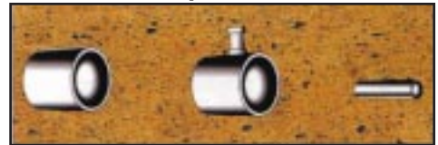
Tracer Wire, Marker Magnet, and Metallic Pipe
